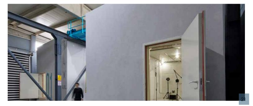
This test method covers the laboratory measurement of airborne sound transmission loss of building partitions such as walls of all kinds, operable partitions, floor-ceiling assemblies, doors, windows, roofs, panels, and other space-dividing elements.
