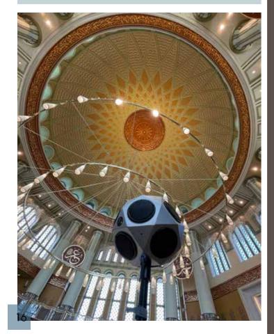
This part of ISO 3382 specifies methods for the measurement of reverberation time in ordinary rooms. It describes the measurement procedure, the apparatus needed, the required number of measurement positions, and the method for evaluating the data and presenting the test report.
